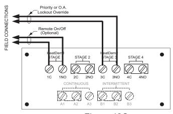
Figure 42C BOILER WITH DOMESTIC HOT WATER PRIORITY OR I/O RESET OVERRIDE
